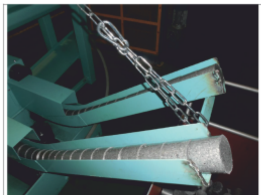
Fig. 5: Briquettes coming out of RUF Press in India
