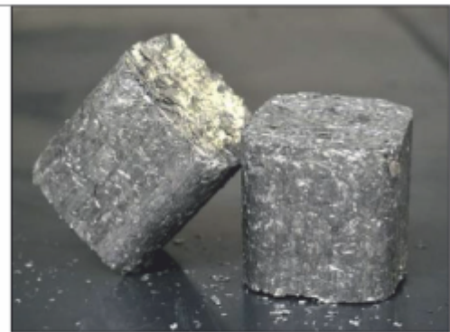
Fig. 4: The 60 x 60 mm sized aluminium briquettes have a higher sales value than loose chips. RUF Maschinenbau GmbH & Co. KG, Germany.
