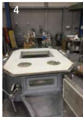
Figure 6: Installation of heating and roof blocks
