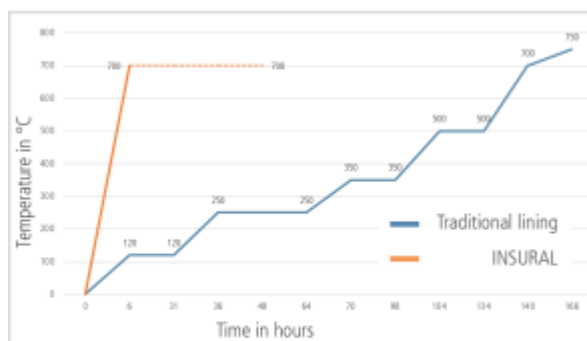
Diagram 1: Comparison of preheating curves
