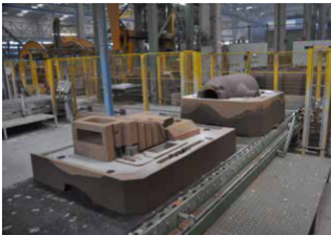
Fig. 3: Assembly of POLISET bonded moulds and POLITEC bonded cores
