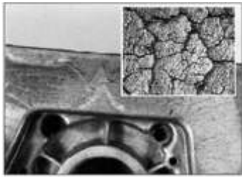
Die Crazing (Thermal Fatigue)
