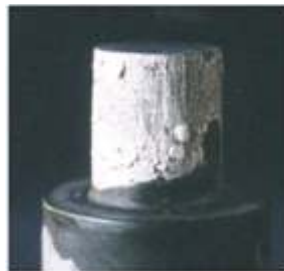
Soldering damage on a core pin.
