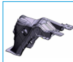
Figure 3: Front wheel shock tower of a passenger car. Initial problems with distortion being out of tolerance after casting and heat treatment were analyzed virtually.
