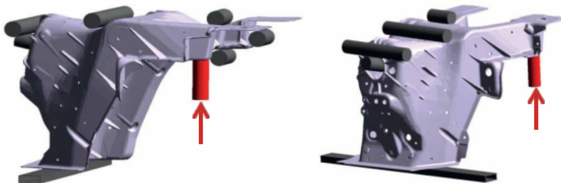
Figure 9: Setup for modeling the straightening process. The dark gray cylinders are constraints and the red cylinder indicates the location and direction of the applied load.
