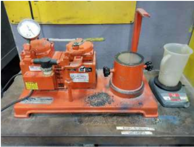
Figure 1. Picture of the RPT apparatus used to assess degassing efficiency.
