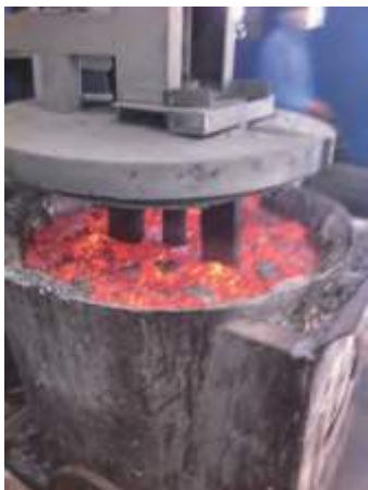
Figure 7. Excessive dross from standard treatment
