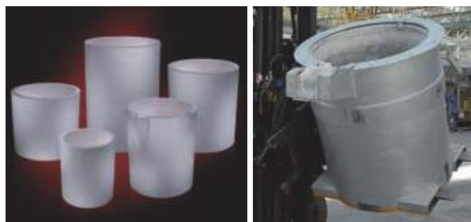
Figure 2. Range of INSURAL 140 lining inserts and INSURALATL in service
