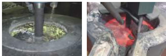
Figure 4. COVERAL MTS 1565 being added into the vortex during MTS 1500 treatment
