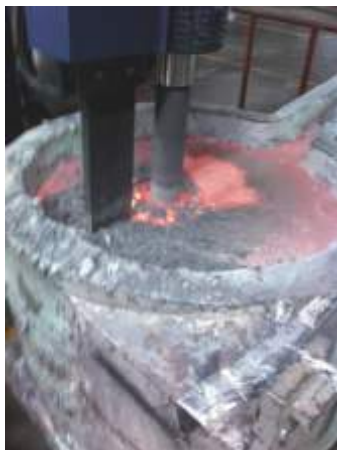
Figure 8. Reduced dross from COVERAL MTS 1565 treatment
