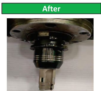
PCD combination tool devolved for Ø 26.1 Boring finishing improved
