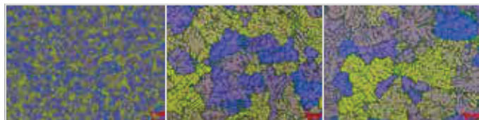
Figure 9b: After treatment. Grain size d_m [ \mu\text{m} ] = 206
