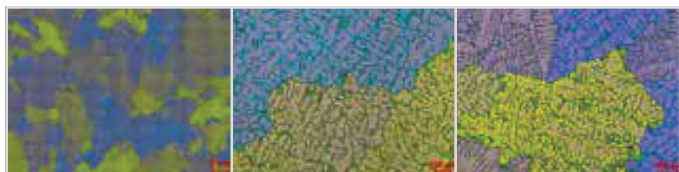
Figure 9a: Before treatment. Grain size d_m [ \mu\text{m} ] = 984
