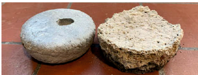
Figure 2: Metal phase and oxide-containing salt phase after dross analysis
