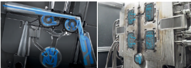
Conformal cooling inserts made by 3D printing
