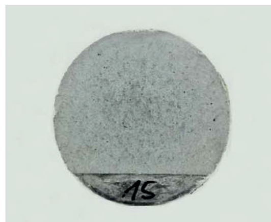
Figure 4: Aluminum sample for SEM examination – after heat treatment
