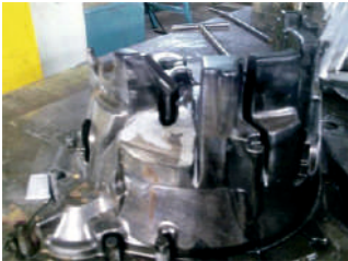
Fracture on the fix side of the die was produced with TOOLOX 44 (After 20,000 cycles' test).
