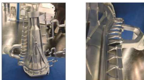
Fig. 11 Gating Design in Large and thin wall casting
