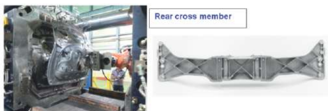
Fig. 5 Example of Large Lightweight Die cast part for Automobile
