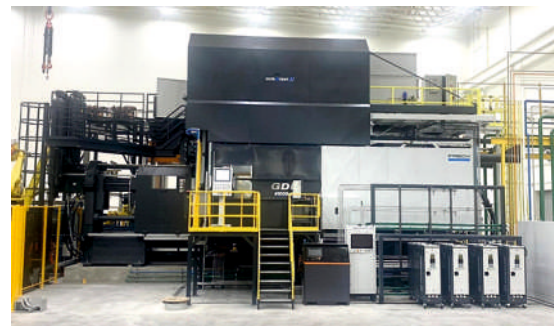
Image: The first model GDK4100S diecasting machine was commissioned
