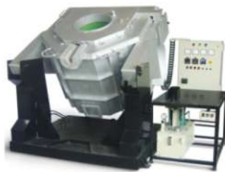
Electrical Hydraulic Tilting Furnace
